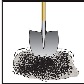
Place **Permanent Asphalt Repair** in hole in layers of 3 inches at a time and tamp the area until firm. The last layer of PAR is to be 25% higher than the finished level.
