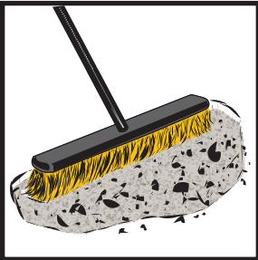
Clean out all loose chunks or debris using a stiff broom or blower to achieve a sound surface to bond to.
