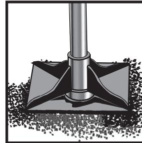
Compact the **Permanent Asphalt Repair** with a tamper, roller or by driving over it until the desired level is obtained.
